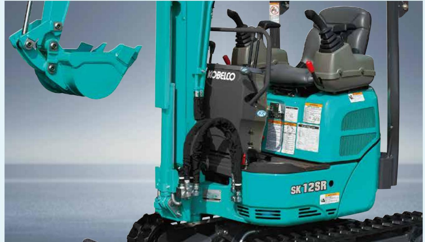
Broader floor space gives operators plenty of foot room. Wide operational space is provided with more room between the left and right control consoles
