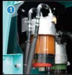
Pre-filter with integrated water separator
