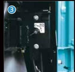
Battery shut-off switch
