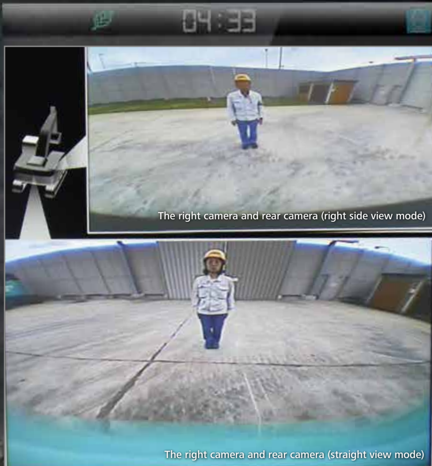
The right camera and rear camera (right side view mode)
