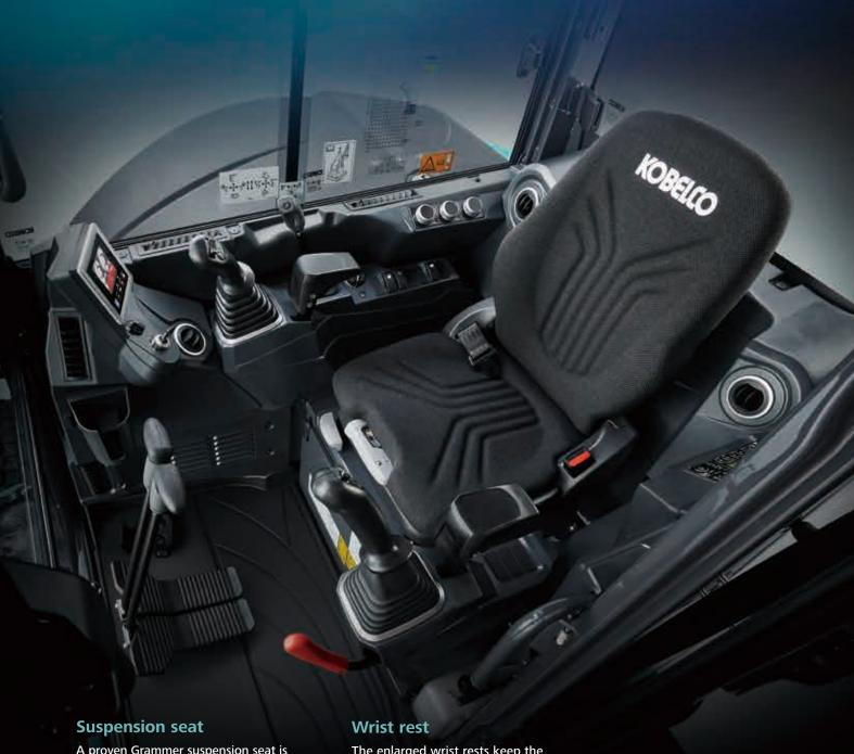
A proven Grammer suspension seat is fitted as standard, offering a reclining mechanism, shock absorber, and excellent seating comfort.
