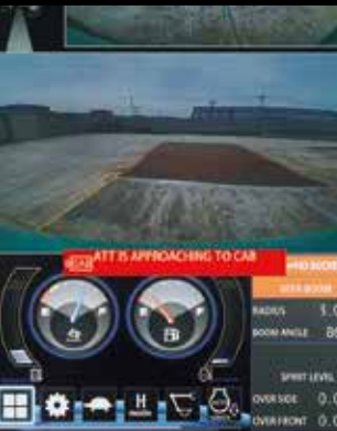
Cab interference warning display
