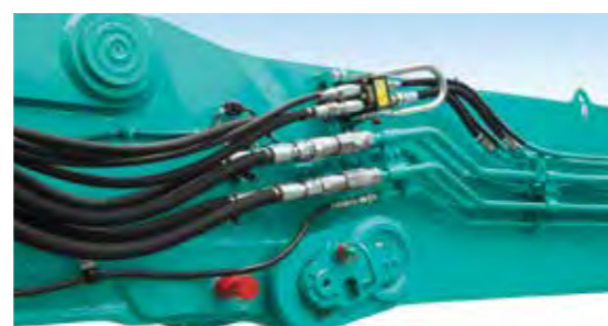
Piping connection: Hydraulic multi-coupler system on the side of the boom.
