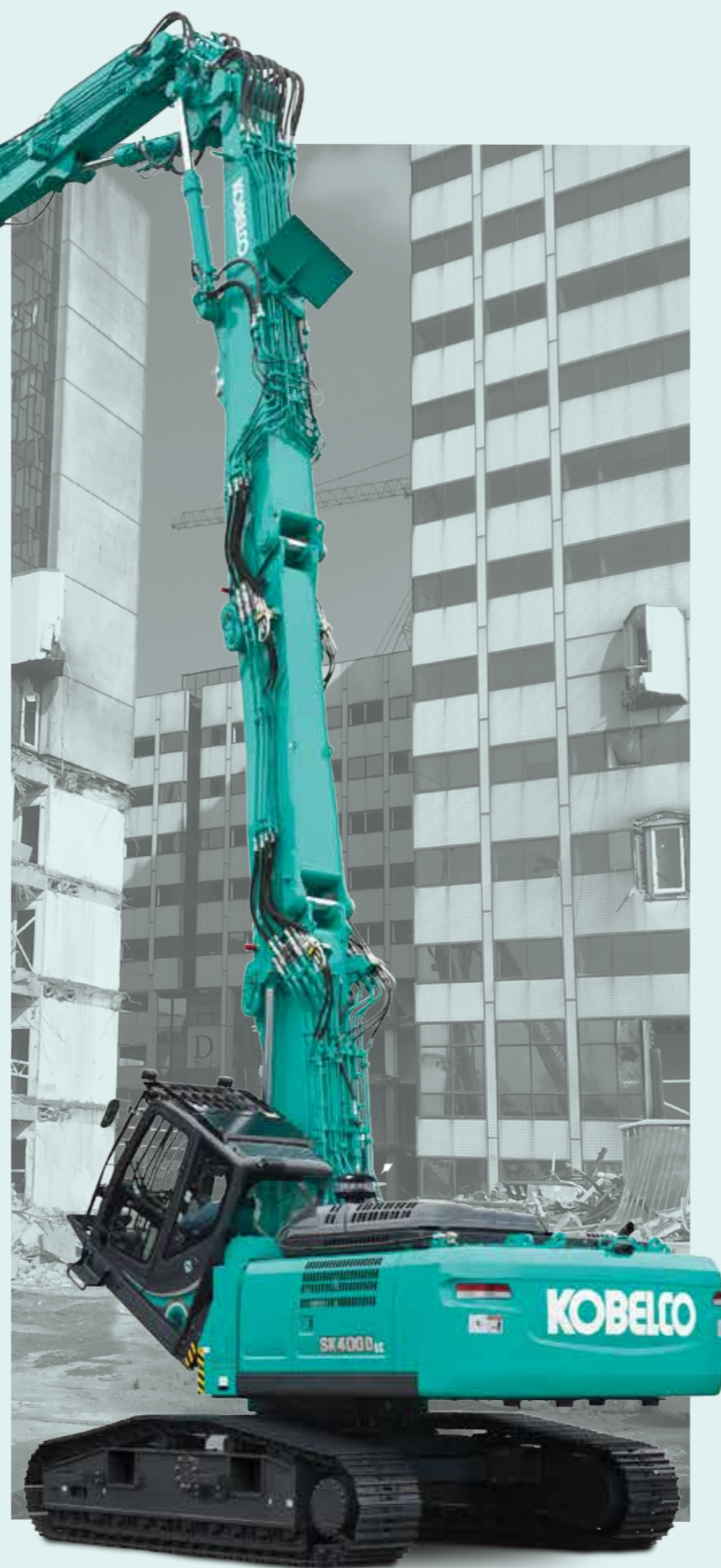
SK400DLC Ultra long attachment specification 6.1m arm + 3.5m boom insert
