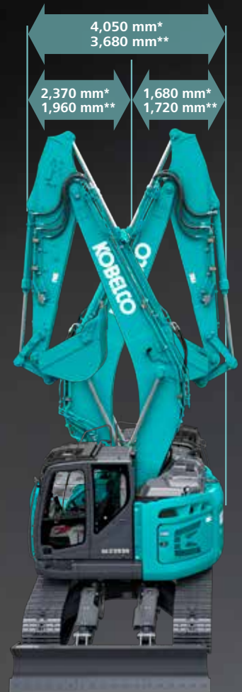
Figures above show the value for standard boom and standard arm spec. * For SK225SR/SK230SRLC ** For SK235SR/SK270SRLC
