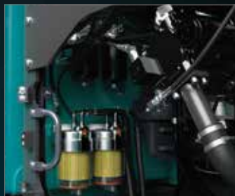
Fuel Filter / Pre-Filter with Integrated Water Separator
