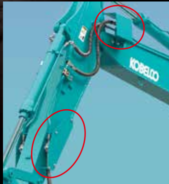
Boom and Arm piping guard (Option)
